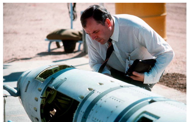
A Soviet inspector examines a BGM-109G Tomahawk ground launched cruise missile (GLCM) prior to its destruction.
